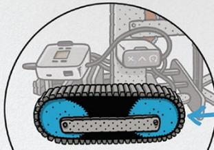
Does it look as though the tank tracks are still in the design? That's the chain drive. It sends power from the motors at the back to the wheels at the front.
